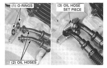
Install the oil cooler to the frame and tighten the bolts securely.
