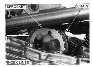
Install the camshaft onto the cylinder head through cam sprocket.
