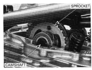
Apply locking agent to the cam sprocket bolt threads. Align the bolt holes in the cam sprocket and camshaft flange and install the cam sprocket bolt.
