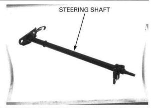
Turn the inner race of steering shaft bearing with your finger.
