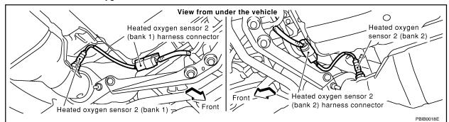
3. Check harness continuity between HO2S2 terminal 4 and ground. Refer to Wiring Diagram.
