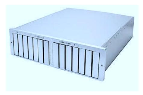
Xserve RAID offers dual independent RAID controllers, up to 14 hot-pluggable hard drives, and two hot-pluggable power supplies. Also featured are several connection options, including dual 2-gigabit fibre channel ports, dual Ethernet ports (for managing the system remotely), and dual uninterruptible power supply (UPS) ports. The system is 5.25 inches (3U) high and can be mounted in a rack with four mounting posts.
