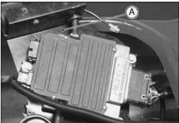
Remove the fuel pump [A] (see Fuel Pump Removal section in this chapter).
