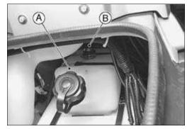
• Remove the bracket [A] holding the EMM, fuel filter and capacitor.
