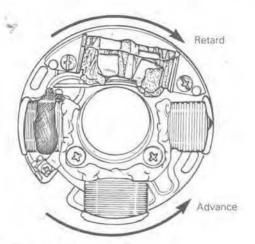
Tighten armature plate screws.
