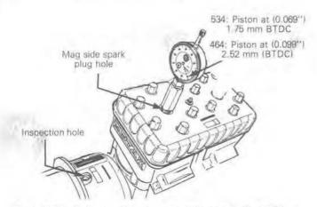
Install dial indicator in magneto side spark plug hole. Bring magneto side piston to top dead center.
