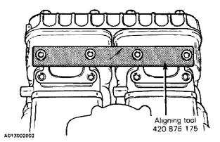
Torque cylinder head nuts to 23 N•m (17 lbf•ft) following illustrated sequence.
